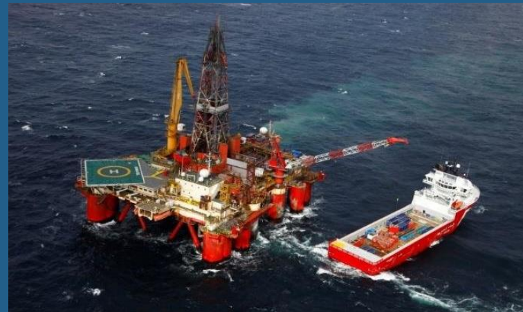
OSV servicing an offshore oil rig
